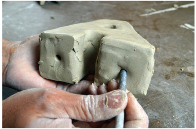
20. Make sure to punch a small hole into the hollow space to keep your letter from exploding in the kiln. You could make the hole on the back of the letter so that you can hang it on the wall or you can hide it on the bottom if your letter will be free standing.
