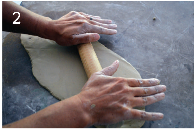
2. Roll out the clay until it is about 10" x 5" long and about 3/8" thick.
