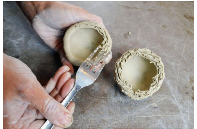
4. Take your scratching tool (wire tool, fork, comb...) and scratch-to-attach the edges of the bowls.
